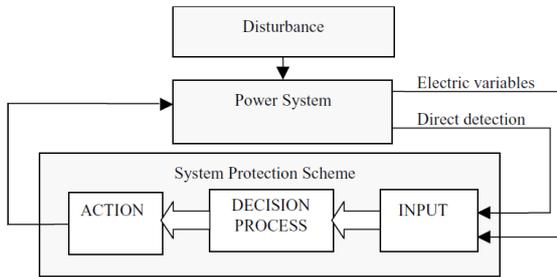
Figure 2: General Structure of a SPS [9]
